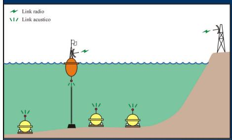
Develop a prototype of seabottom wire-less system of seismic data acquisition and transmission using acoustic link and electro-acoustic sensor technology
